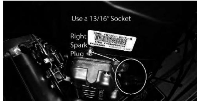
2) Check the gap on the spark plug to verify that it is 0.03 in using a feeler gauge.
