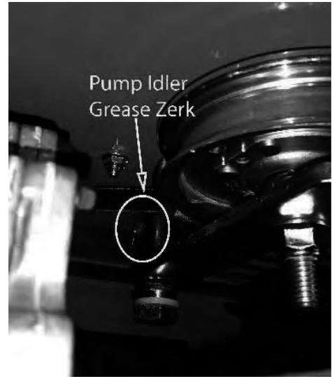
The deck belt tensioner is located at the rear of the deck and has a grease fitting on its pivot point. Grease at every engine oil change.
