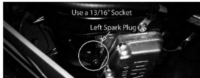
4) Install the plug into cylinder head and torque to 16 ft.-lbs. Be careful not to overtighten the spark plug.
