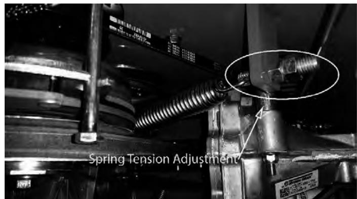
Use a belt tension gauge to ensure the proper tension. Your dealer or service center will have a belt tension gauge or you can buy one (Part Number 041-9999-00).
