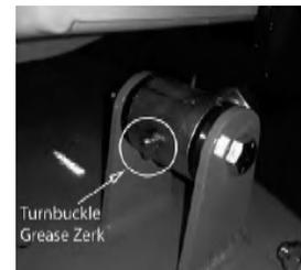
The pump belt tensioner is located under the engine and has a grease fitting at its pivot point. Grease at every engine oil change.
