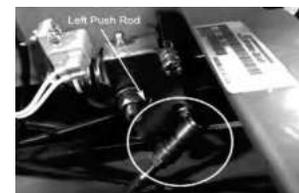
When adjusting the tracking on the mower, the length of the pushrods can be changed by screwing the pivot joint in or out on the ends of the rods. Shortening the overall length of the rod slows the pump down. Lengthening the rod will increase the speed of the pump.
