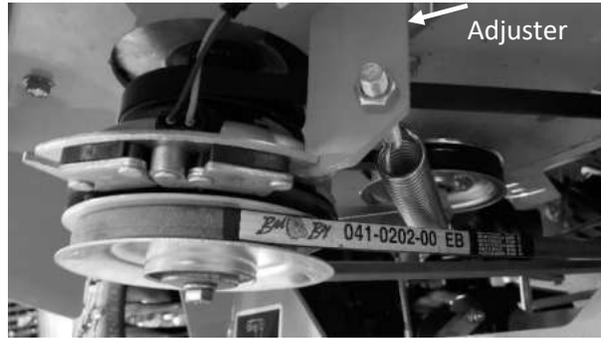
The tension should be adjusted so that there is between 60 to 65 lbs. of tension on the belt. This can be checked with a belt tension gauge as shown to the right.
