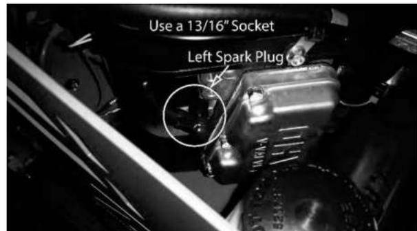
3. If the spark plug is worn, overheated, wet, or carbon fouled replace the spark plug.
